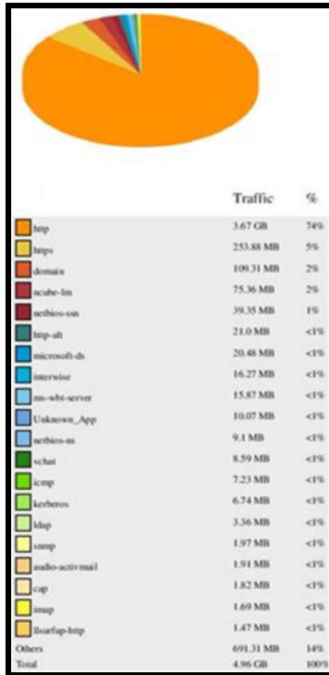
Figure 4.5: Percentage of traffic usage. (c) Percentage of traffic usage of applications/protocols in one branch network.
